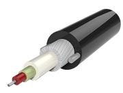
Fiber OSP cable, A2 Dual-sheathed HDPE Drop, LSZH Subunit, Loose buffer, Singlemode, G.657.A2, 1 fiber, Gel-filled, Meters jacket marking, Black jacket color
