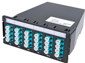
Universal Connectivity Platform (UCP) Q-Fit Module, 2xMPO to 6xLC-quad, OM3, pair flipped
