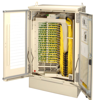
FDH 3000 Small Fiber Distribution Pole Mount Cabinet, 288F, SC/APC,(2) 32-splitter module, die. loose tube, 200 ft, 48F
