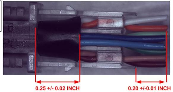
Push cable jacket to dimension 0.25 +/- 0.02 inch. Cut wires to dimension 0.20 +/- 0.01 inch.
