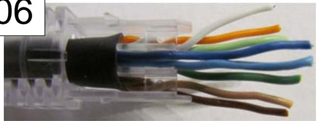
Untwist all wire pairs and **Add Twist** to **Orange** and **Brown** pairs to align with Step 7. Make sure **No Twist** in **Blue** and **Green** pairs back to jacket.
