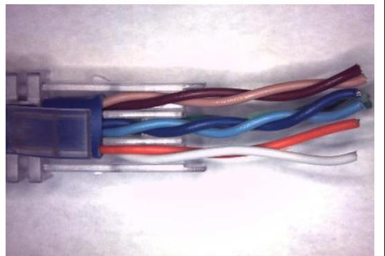
On reverse latch side wire pairs; **Orange**, **Blue**, and **Brown** are positioned as shown.
