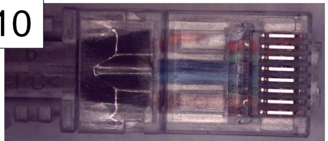
Push the plug housing over the load bar through the boot pair manger all the way until it latches to the boot. Terminate plug contacts to wire pairs with termination tool to seat the contacts.
