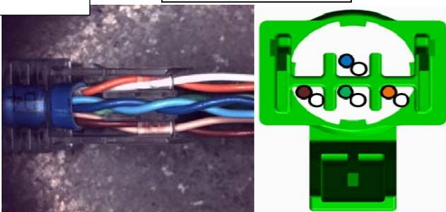
Insert cable jacket and wire pairs into boot/pair manager with **Blue** wire pair on top.
