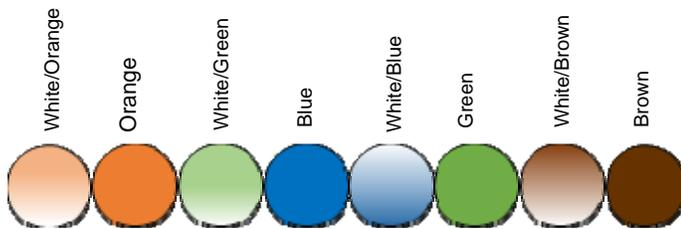
Align wires to standard T568B wiring pattern.
