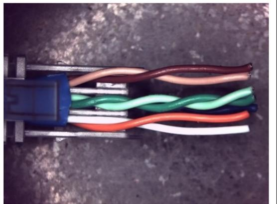
On the reverse latch side; **Orange**, **Green**, and **Brown** wire pairs are positioned as shown.
