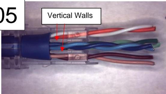
Slide boot/pair manager down to cable jacket (see step #8). Ensure vertical walls are wedged in-between wire pairs as shown.
