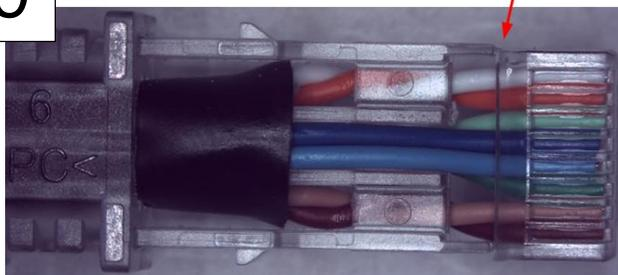
Slide wire pairs into load bar until wire insulation reaches ending point. Make sure wires are all the way into load bar housing.
