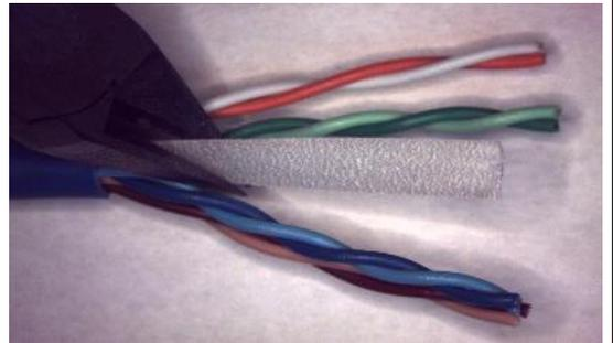
Cut away filler strip from end of cable jacket. Cut as close as you can to the edge of the cable jacket without nicking wires insulation.
