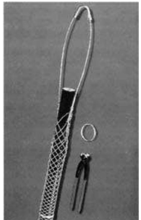
*Figure 2: A non-laced hoisting grip is a one-piece unit that slips over the transmission line and applies tension to prevent slippage during and after installation. This support/hoisting grip is shown with the calibrated clamp that locks the grip into place and with the crimping tool for installing the clamp.*
