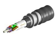
Fiber indoor/outdoor cable, TeraSPEED®, Plenum Rated, 144 fiber, Singlemode G.652.D and G.657.A1, Gel-Free, Stranded Loose Tube with Aluminum Interlocking Armor containing a Plenum Rated Outer Jacket, Black jacket color, Feet cable marking
