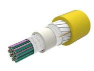
Fiber indoor cable, All-Dielectric, LSZH/Riser-Rated, Gel-Free, Central Tube 200µm Rollable Ribbon, 288 fiber, Singlemode G.657.A2/B2, Feet jacket marking, Yellow jacket color, Cca flame rating
