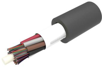
Fiber indoor/outdoor cable, LightScope® ZWP Low Smoke Zero Halogen, 96 fiber Microsheath, OM5 , Gel-free, Meters jacket marking, Black jacket color, B2ca flame rating
