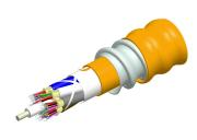
Fiber indoor cable, OptiSPEED® Plenum Distribution, interlocking aluminum armored with plenum jacket, 6 fiber single-unit, Gel-free, Multimode OM1, Feet jacket marking, Orange jacket color
