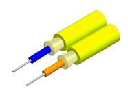
Fiber Indoor Cable, 1.6mm Low Smoke Zero Halogen Riser, 2-fiber Zipcord, Singlemode G.652.D and G.657.A1, Feet jacket marking, Yellow jacket color, Eca Flame Rating
