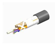
Fiber indoor/outdoor cable, LazrSPEED®, Single Jacket All-Dielectric, Plenum Rated, Multimode OM4, Gel-Free, 144 fiber, Stranded Loose Tube, PVDF jacket, Black jacket color, Feet cable marking
