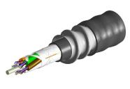
Fiber indoor/outdoor cable, TeraSPEED®, Plenum Rated, Singlemode G. 652.D and G.657.A1, Gel-Free, 12 fiber, Stranded Loose Tube with Aluminum Interlocking Armor containing a Plenum Rated Outer Jacket, Black jacket color, Feet cable marking
