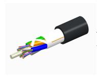
Fiber indoor/outdoor cable, LazrSPEED®, Single Jacket All-Dielectric, Low Smoke Zero Halogen (LSZH), 24 fiber, Gel-Free, Stranded Loose Tube, Multimode OM3, Black jacket color, Custom cable marking, Eca flame rating
