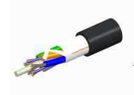
Fiber OSP cable, LazrSPEED® Single Jacket All-Dielectric, 144 fiber, Gel-Free, Stranded Loose Tube, Multimode OM4, Feet jacket marking, Black jacket color
