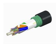
Fiber OSP cable, TeraSPEED® Single Jacket/Single Armor, Gel-Free, 96 fiber, Stranded Loose Tube, Composite OM4 and G.652.D and G.657.A1, Feet jacket marking, Black jacket color
