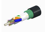
Fiber OSP cable, TeraSPEED® Single Jacket/Single Armor, 252 fiber, Gel-Free, Stranded Loose Tube, Singlemode G.652.D and G.657.A1, Feet jacket marking, Black jacket color
