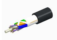
Fiber OSP cable, TeraSPEED® Single Jacket All-Dielectric, Gel-Free, Stranded Loose Tube, 24 fibers, Composite OM4 and G.652.D and G.657. Al, Feet jacket marking, Black jacket color
