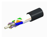
Fiber OSP cable, TeraSPEED® Single Jacket All-Dielectric, 72 fiber, Gel-Free, Stranded Loose Tube, Singlemode G.652.D and G.657.Al, Feet jacket marking, Black jacket color
