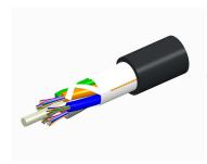
Fiber OSP cable, TeraSPEED® Single Jacket All-Dielectric, 36 fiber, Gel-Free, Outdoor Stranded Loose Tube w/HDPE Outer Jacket, Singlemode G.652.D and G.657.Al, Feet jacket marking, Black jacket color
