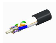
Fiber OSP cable, TeraSPEED® Single Jacket All-Dielectric, Gel-Free, 12 fibers, Stranded Loose Tube, Composite OM4 and G.652.D and G.657.Al, Feet jacket marking, Black jacket color
