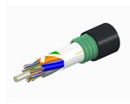
Fiber OSP cable, TeraSPEED® Single Jacket/Single Armor, Gel-Free, 8 fibers, Stranded Loose Tube, Singlemode G.652.D and G.657.A1, Feet jacket marking, Black jacket color
