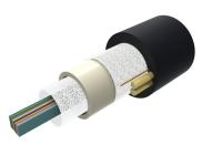
Fiber OSP Cable, Non-Armored, All-Dielectric, 432 fiber, Arid-Core, Dry Central Tube Ribbon, Singlemode G.652.D and G.657.Al, Gel-free, Feet jacket marking, Black jacket color
