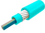
Fiber Indoor Cable, Multimode OM3 bend insensitive, 36 fibers, Plenum, All-Dielectric Central Tube Ribbon, Gel-free, Feet jacket marking, Aqua jacket color
