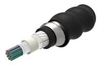
Fiber indoor/outdoor cable, Interlocking Armored, LSZH Riser-Rated, 144 fiber, Gel-Free, Central Tube Rollable Ribbon, Singlemode G.657.A2/B2, Feet jacket marking, Black jacket color, B2ca flame rating
