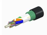
Fiber indoor/outdoor cable, TeraSPEED®, Single Jacket/Single Armor, Low Smoke Zero Halogen (LSZH), 24 fiber, Singlemode G.652.D and G. 657.A1, Gel Filled , Stranded Loose Tube, Black jacket color, Meters jacket marking, Cca flame rating
