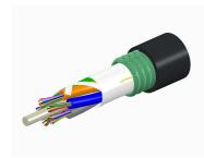
Fiber indoor/outdoor cable, TeraSPEED®, Single Jacket/Single Armor, Low Smoke Zero Halogen (LSZH), 96 fiber, Singlemode G.652.D and G. 657.A1, Gel Filled, Stranded Loose Tube, Black jacket color, Meters jacket marking, Cca flame rating
