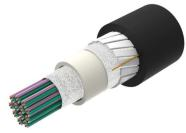
Fiber indoor/outdoor cable, All-Dielectric, LSZH Riser-Rated, Gel-Free, Central Tube Rollable Ribbon, 216 fiber, Singlemode G.652.D and G.657. Al, Feet jacket marking, Black jacket color, Cca flame rating
