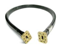
FlexTwist® Flexible Twist for WR112, 7.05–10.0 GHz, with interface types UBR84 and UBR84, 600 mm
