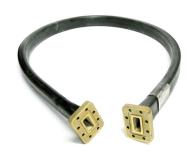
FlexTwist® Flexible Twist for WR137, 6.425–7.125 GHz, with interface types CPR137G and CPR137G, 1200 mm
