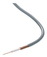
FSJ1-75A, HELIAX® Superflexible Foam Coaxial Cable, corrugated copper, 1/4 in, gray non-halogenated, fire retardant polyolefin jacket
