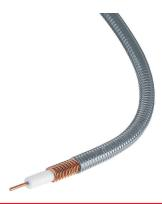
FSJ4-75A, HELIAX® Superflexible Foam Coaxial Cable, corrugated copper, 1/2 in, gray non-halogenated, fire retardant polyolefin jacket
