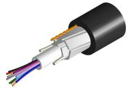
Fiber Indoor/Outdoor Drop Cable, LazrSPEED®, Low Smoke Zero Halogen Single Jacket All-Dielectric Arid-Core, 12 fiber, Gel-filled, Multimode OM3, Feet jacket marking, Black jacket color, Dca flame rating
