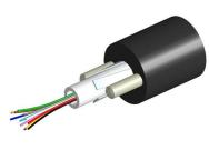
Fiber drop cable, LazrSPEED® Single Jacket All-Dielectric Arid Core, 4-fiber, Multimode OM3, Gel-filled, Feet jacket marking, Black jacket color
