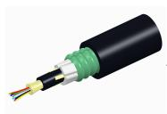
Fiber outdoor drop cable, Low Smoke Zero Halogen Single Jacket Single Armor Arid-Core, Singlemode G.657.A2/B2, Gel-free, Feet jacket marking, Black jacket color
