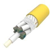
Fiber indoor cable, All-Dielectric, LSZH Riser-Rated, Gel-Free, Loose Tube Rollable Ribbon, 1728 fiber, Singlemode G.657.A2, Feet jacket marking, Yellow jacket color
