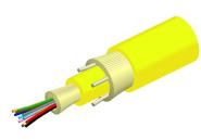
Fiber indoor cable, Low Smoke Zero Halogen Riser MPO Trunk with 2.0 mm Subunits, 8 fiber, Singlemode G.657.A2/B2, Feet jacket marking, Yellow jacket color, Dca flame rating
