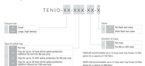
TENIO-C6H accommodates up to 12 trays; each tray houses 24 fiber splices for a capacity of 288 fibers.
