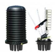
FOSC® 400 A8 Fiber Optic Splice Closure, Heat Shrink Cable sealing, one pre-installed 12-splice tray, ground feedthrough lugs, with test valve
