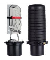
FOSC® 450 A4 Fiber Optic Splice Closure, Gel Cable sealing, one pre-installed 12-splice tray, 2 cable attach., one ground feedthrough lug, with test valve
