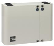
FL1000 Fiber Wall Box, 2-door, singlemode SC/UPC, 12-ports, with pigtails and splice tray, 1 cable clamp, 1 compression fitting, 1 strength member tie-off, 1 key lock
