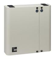
FL1000 Fiber Wall Box, 2-door, singlemode SC/APC, 24-ports, with pigtails and splice tray, 1 cable clamp, 1 compression fitting, 1 key lock
