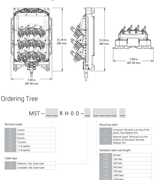
\*0-300 ft lengths of cable is automatically coiled (option U), for greater than 300 ft cable lengths, choose U or A option.
