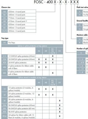
V Pre-installed flash test valve N No flash test valve Ground feedthrough © Pre-installed ground feedthrough N No ground feedthrough
