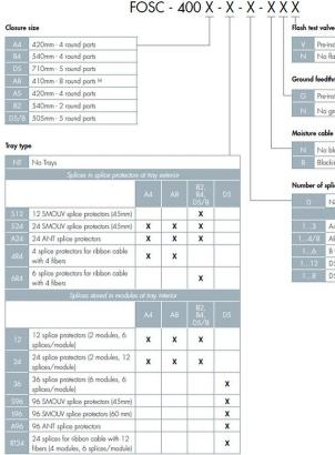
Pre-installed flash test valve No flash test valve Ground feedthrough G Pre-installed ground feedthrough N No ground feedthrough
