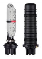
FOSC® 400 B4 Fiber Optic Splice Closure, Heat Shrink Cable sealing, no pre-installed trays, cable blocking, ground feedthrough lugs, with test valve
