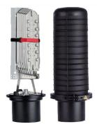
FOSC® 450 D6 Fiber Optic Splice Closure, Gel Cable sealing, one preinstalled 36-splice tray, 6 cable attach., tall, 3 ground feedthrough lugs, with test valve
