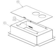
FDH Pad Mount Frame for small sized shells (FDH3000 FD3-AC\* and FDH5000 Models)
