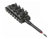
DLX® Mini-MST, Fiber Optic Multiport Service Terminal, 8-port with 1x8 splitter, dielect. flat loose tube cable, 350 ft
