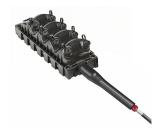
DLX® Mini-MST, Fiber Optic Multiport Service Terminal, 8-port with 1x8 splitter, dielect. flat loose tube cable, 610 m
