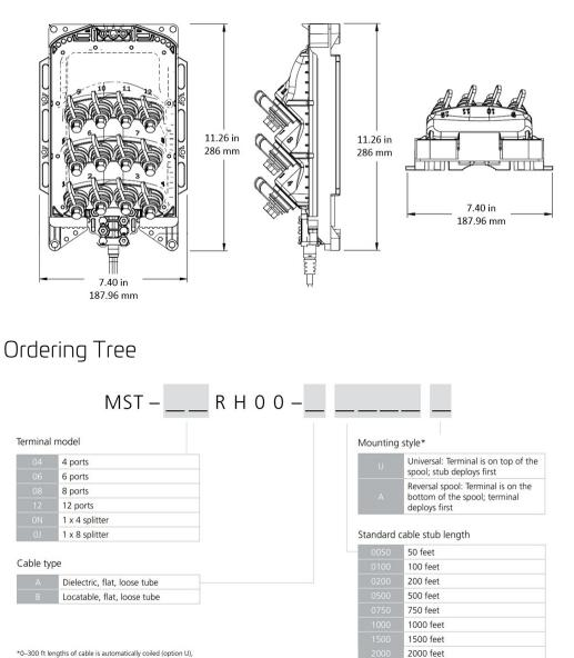
\*0-300 ft lengths of cable is automatically coiled (option U), for greater than 300 ft cable lengths, choose U or A option
